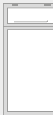
GLASS TO GROUND WINDOW WIDE WITH TOP LITE WIDTH- 745MM HEIGHT- 1755MM WCT15 TOP HUNG TOP LITE
