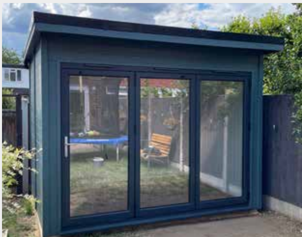
10' X 8' Pent garden studio, thermowood cladding, Aluminium 3 leaf 9ft bifold doors anthracite grey, MDF (V grooved) painted lining (white) with breathable membrane (moisture barrier) and Celotex insulation, painted finish in anthracite grey, EPDM rubber roof, laminate floor in classic oak & black guttering
