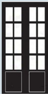
8 PANE WIDTH - 1155MM HEIGHT - 1858MM WG8
