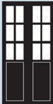
6 PANE WIDTH - 1155MM HEIGHT - 1858MM WG6
