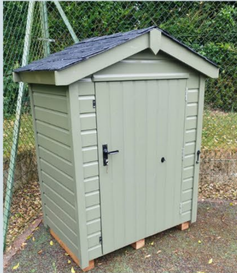
4' x 2'6" Mini Shed Apex -pressure treated timber, heavy duty cladding, slate effect tile roof, painted finish olive, 2' 9" single door with security upgrade, bearers
