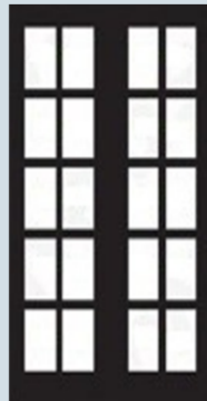
10 PANE WIDTH - 1155MM HEIGHT - 1858MM WG10
