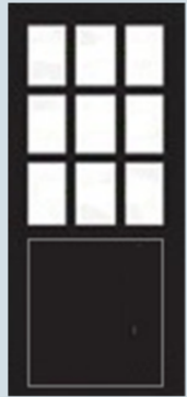
9 PANE WIDTH - 815MM HEIGHT - 1858MM WG9
