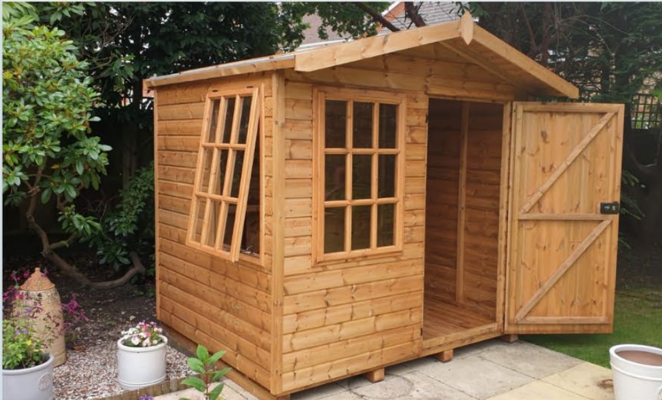
7'6" x 6' Heritage Chalet Apex - pressure treated timber, heavy duty cladding, solvent treated, single shed door, 2 fixed 9 pane georgian windows to front, 2 additional 9 pane georgian top hung opening windows to sides, black fittings, bearers, toughened glass, felt roof
