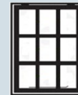
9 PANE WIDTH - 745MM HEIGHT - 1060MM Top hung only WGS9
