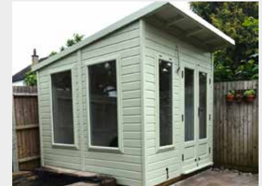
7'6" X 8' Heritage Summerhouse Pent - Painted finish thyme, painted MDF lining & insulation white, EPDM rubber roof, 3/4 length straight top double doors & windows (1 top hung narrow to front & 2 fixed wide windows to one side), double glazed, black fixings, veneto oak laminate flooring, fit customer cables, solvent treatment to roof & floor, bearers, tanalised timber & heavy duty cladding
