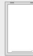
3/4 LENGTH WINDOW WIDE WITH SASH WIDTH- 745MM HEIGHT- 1375MM WCS12 TOP HUNG ONLY
